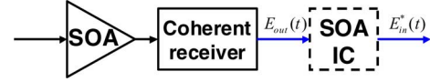
Fig. 1. Diagram of a single SOA IC. Optical path: black line. Electrical path: blue line.
