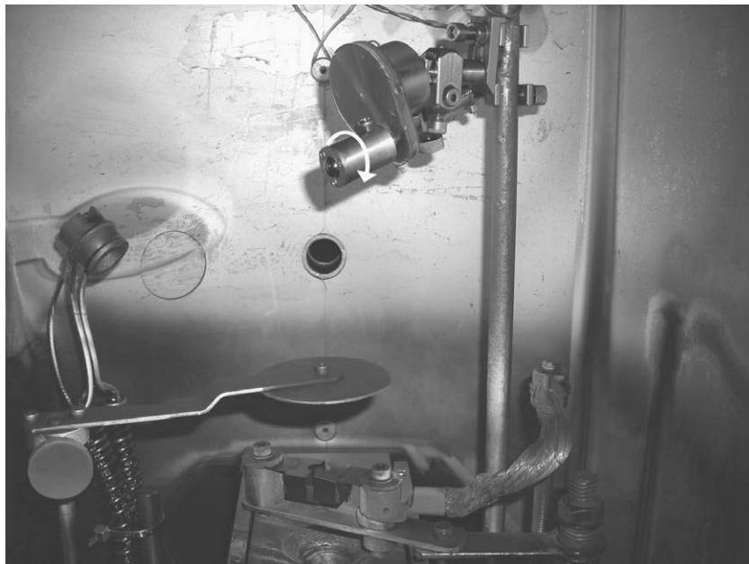
Fig. 1. Photograph of the rotating device inside evaporation chamber. The hemispherical lens is located 14 cm directly above the thermal boat and rotated in the direction indicated by the white arrow.
