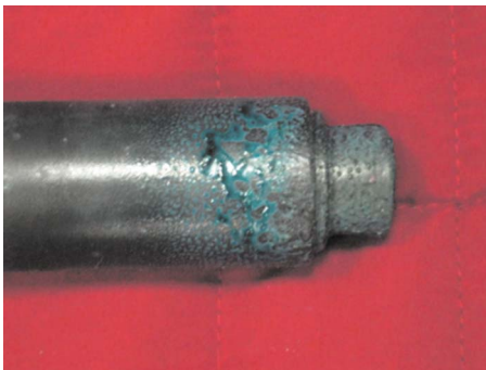
Fig. 16 Probe condition showing copper sulfate deposits after 28 continuous days in the rig (available in color online)
