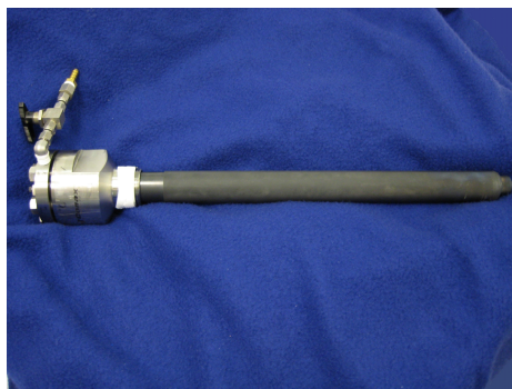
Figure 2. All-SiC temperature frontend probe shown in an assembled fashion.
