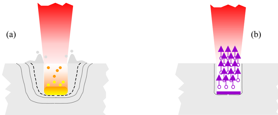
Fig.1. Schematic illustrating the difference between (a) conventional and (b) femtosecond micromachining
