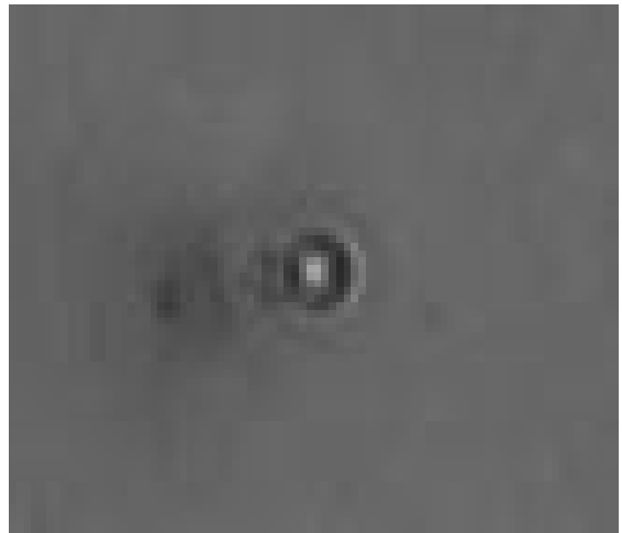
Fig. 8. Cross section of a longitudinal waveguide written in bulk 90%(GeS 2 )-10%(Sb 2 S 3 )
