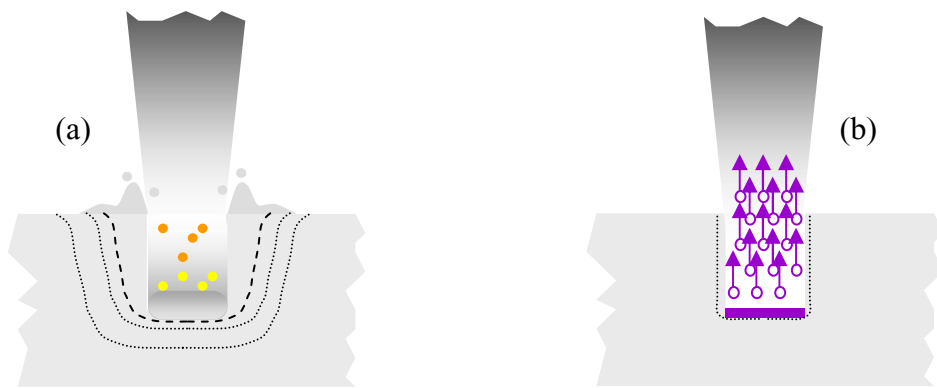
Figure 1 – Schematic illustrating the difference between conventional (a) and femtosecond (b) micromachining
