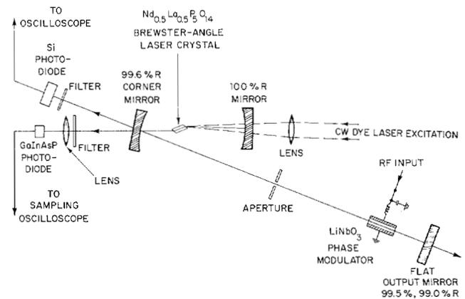
Fig. 1. Schematic diagram of FM mode-locked Nd<sub>0.5</sub>La<sub>0.5</sub>P<sub>5</sub>O<sub>14</sub> laser.
