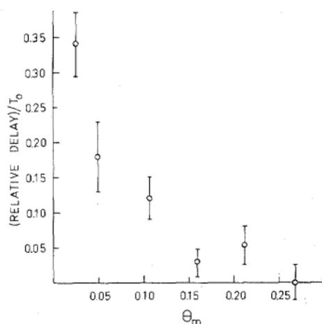
Fig. 9. Relative delay of the pulse, normalized to the interpulse separation, as a function of the modulation index  $\theta_m$ .
