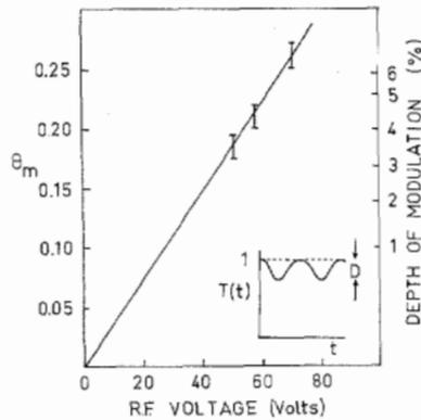
Fig. 2. Relationship between the depth of modulation  $D$  and  $\theta_m$  and the deduced RF voltages that were applied. The inset shows how  $D$  was defined.
