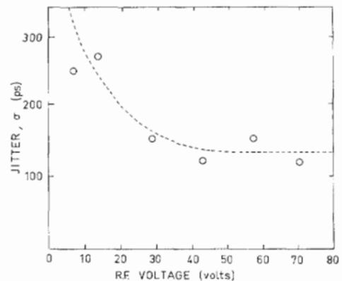
Fig. 8. Jitter as a function of applied RF voltage.
