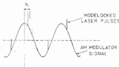
Fig. 6. Schematic diagram illustrating how the jitter was determined.
