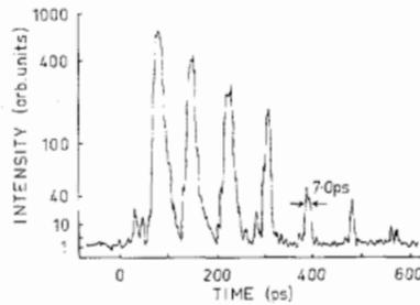
Fig. 5. Pulsewidth when only passive mode locking was applied.
