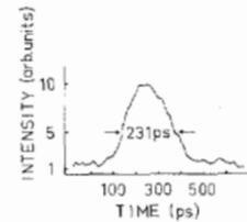
Fig. 3. Pulsewidth when only active mode locking was applied.
