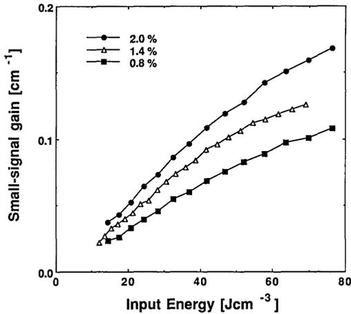
Fig. 3. Small-signal gain at 850 nm versus electrical input energy in  $\text{LiSrAlF}_6:\text{Cr}^{3+}$  for  $\pi$ -polarized light for three different  $\text{Cr}^{3+}$  concentrations.
