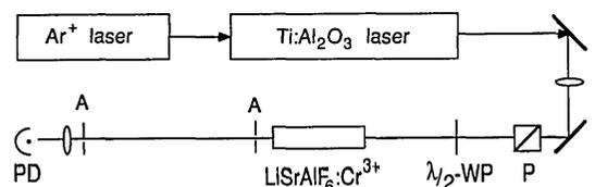
Fig. 1. Experimental setup. P, polarizer; WP, wave plate; A's, apertures; PD, photodiode.
