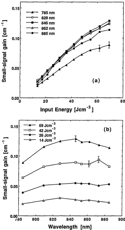
Fig. 2. Small-signal gain (a) versus electrical input energy and (b) versus wavelength in  $\text{LiSrAlF}_6:\text{Cr}^{3+}$  for  $\pi$ -polarized light.
