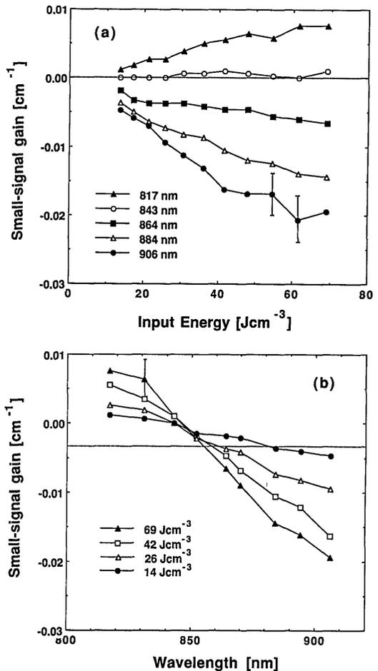
Fig. 4. Small-signal gain (a) versus electrical input energy and (b) versus wavelength in  $\text{LiSrAlF}_6:\text{Cr}^{3+}$  for  $\sigma$ -polarized light.
