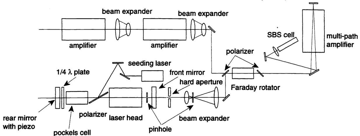
Fig.1 A compact tabletop type glass laser system with injection seeded oscillator, multi-path amplifier, and SBS phase conjugat mirror. This laser system provides a 20J and 10ns pulse.
