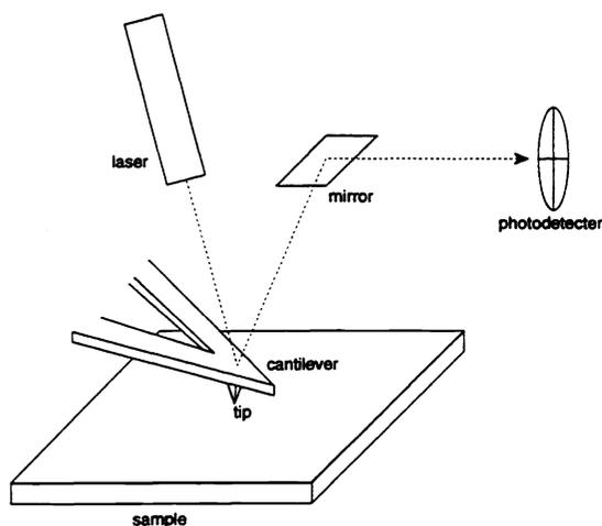
Fig.4 A schematicview of the AFM.
