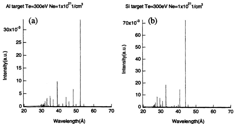
Fig.2 Typical x-ray line emissions from (a) Al and (b) Si calculated with RATION code. Electron temperature 300eV and electron density  $1 \times 10^{21} \text{ 1/cm}^3$  are used.
