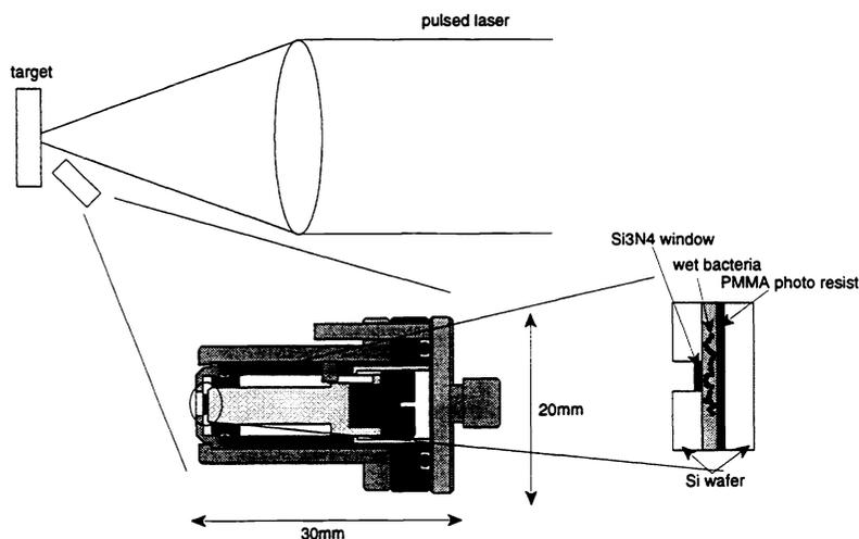
Fig.3 Experimental setup and a schematic view of a sample holder. A pulsed laser is focused to produce plasmas. The sample holder is placed 1cm to 2cm from target.
