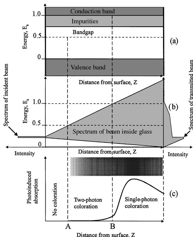
Fig. 5. Photoinduced processes in a dielectric material exposed to femtosecond IR pulses.
