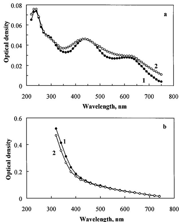
Fig. 2. Spectra of additional absorption of a, high-purity alkali silicate glass and b, K8 borosilicate glass exposed to 1,  $\gamma$  radiation or 2, femtosecond laser radiation at 850 nm. The thickness of both samples was 6 mm.
