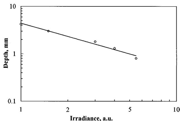
Fig. 4. Dependence of the distance between the front surface of the sample and the colored region (depth, marked A in Figs. 1 and 3) on the irradiance of the incident laser radiation. The solid line is a hyperbolic curve:  $y \propto x^{-0.93}$ .
