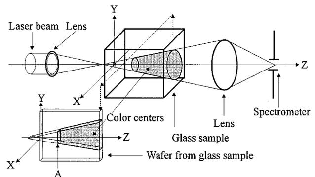
Fig. 1. Experimental setup for exposure of glass samples to IR femtosecond laser pulses, measurement of spectra and spatial distribution of photoinduced absorption, and measurement of spectra of emitted radiation.
