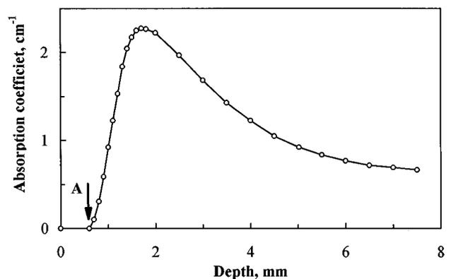
Fig. 3. Dependence of the additional absorption coefficient on the distance from the front surface of K8 glass (depth, axis  $Z$  in Fig. 1) irradiated by femtosecond laser radiation at 850 nm. The lens focal length was 100 cm; the sample thickness was 2 cm.
