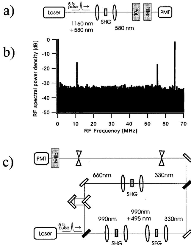
QFC2 Fig. 2. a) Interference between fundamental and second harmonic in a compact detector. Second harmonic light interferes with the other end of the fundamental spectrum in a polarizer. A PMT detects the beat frequency. b) The resulting RF-spectrum. c) Interference between the second and the third harmonics in a Mach-Zehnder type interferometer
