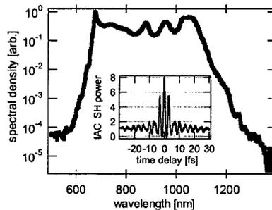
QFC2 Fig. 1. Octave spanning power spectrum directly from the two-foci-laser-oscillator on a logarithmic scale. Inset: Interferometric autocorrelation; a phase retrieval algorithm reveals a pulse FWHM of 5.0 fs.
