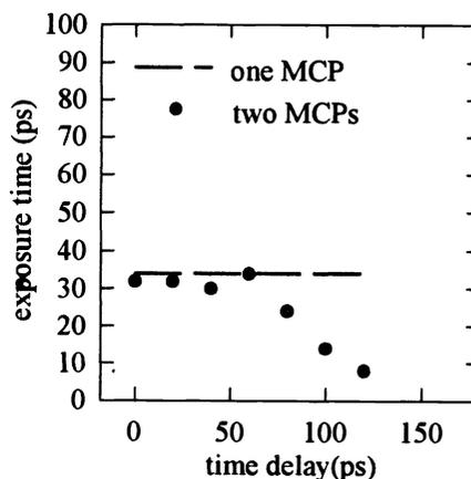
**Fig. 8(b)** The exposure time vs. the time delay for MCPs gated by 75 ps pulses
