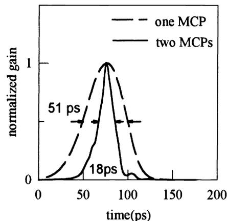
**Fig. 9 Comparison of the exposure time of one MCP with two MCPs gated by 100 ps pulses**
