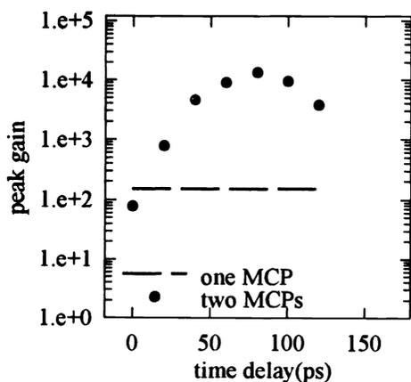
**Fig. 8(a)** The peak gain vs. the time delay for MCPs gated by 75 ps pulses
