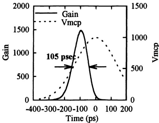
**Fig. 3** The dynamic gain of the MCP gated by the voltage pulse whose FWHM is 300 ps
