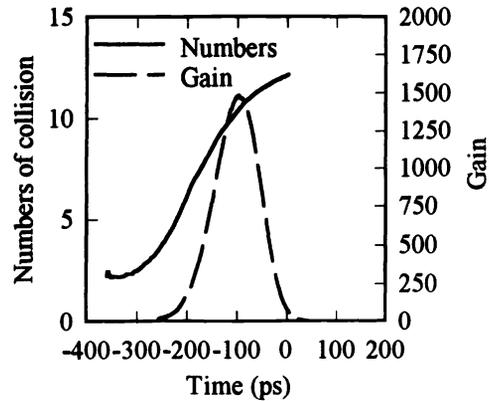
**Fig. 4** Numbers of electron collision on the wall of the MCP gated by the voltage pulse of 300 ps
