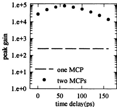
**Fig. 7(a)** The peak gain vs. the time delay for MCPs gated by 150 ps pulses
