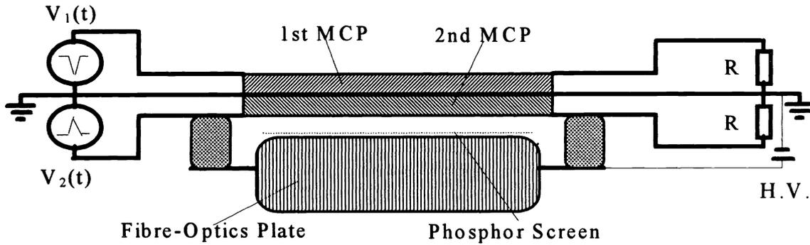
**Fig.1 Principle of gating two MCPs in cascade**
