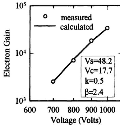
**Fig. 2** Calculated MCP gain vs voltage(solid lines) and measured data (plotted points) at  $V_1=800$  Volts for MCP of  $\alpha=40$  and  $\phi=10$
