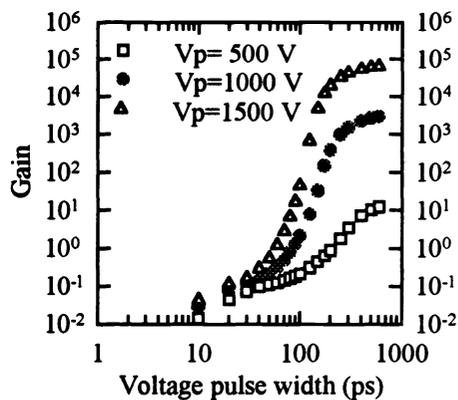
**Fig. 6** Peak gain vs. the width of the voltage pulse whose peak amplitude is  $V_p$
