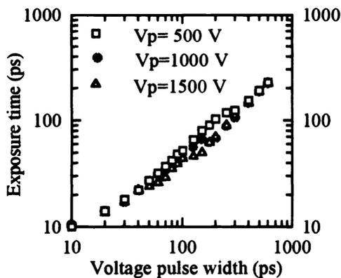
**Fig. 5** Exposure time vs. the width of the voltage pulse whose peak amplitude is  $V_p$ .
