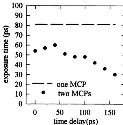
**Fig. 7(b)** The exposure time vs. the time delay for MCPs gated by 150 ps pulses
