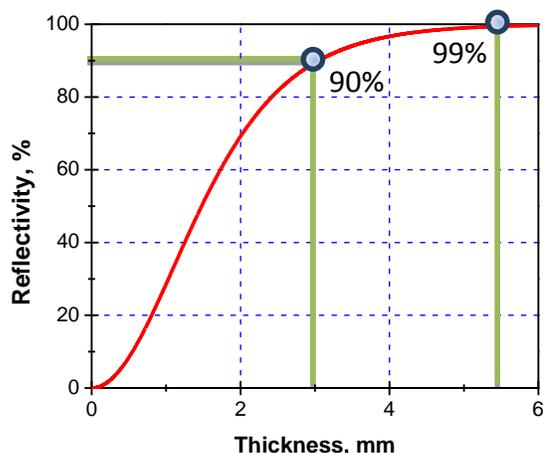
Figure 8: VBG reflectivity dependence on thickness
