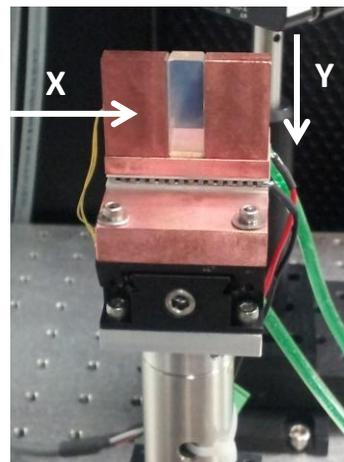
Figure 7: Double MBVG thermal stability control mounting
