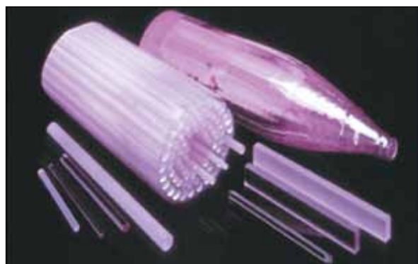
Single laser crystals grown by conventional Czochralski growth are limited by boule size and corable rod diameters, typically a few centimeters.
