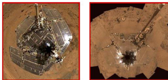
Fig 1. Comparison view of the clean solar panels and the rover almost blended into the dusty background on Mars [7]
