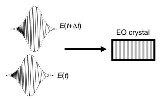
Fig. 4. Scheme to generate tunable THZ radiation from the overlap of two linearly chirped pulses.
