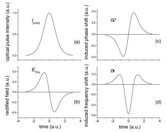
Fig. 7. (a) The optical pulse intensity profile, (b) rectified field profile, (c) phase profile across the optical pulse after traveling the crystal, and (d) frequency shift of the optical pulse.
