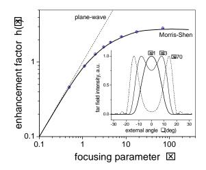
Fig. 5. Enhancement factor *h* as a function of the focusing parameter  $\xi$ . Solid curve is based on ref. 22. Dashed curve – plane-wave approximation. Dots represent our calculations based on the Green's function method. Inset: far field THz intensity profiles at different  $\xi$  for a 1-cm-long GaAs.
