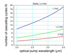
Fig. 6. Number of THz cascading cycles as a function of THz frequency and pump wavelength for GaAs, L=1 cm.
