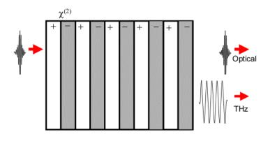
Fig. 1. Illustration of optical rectification in a media with periodically inverted  $\chi^{(2)}$  sign, using femtosecond pump pulses. The static picture shows optical and THz electric fields, while the animation shows the nonlinear driving polarization and the THz electric field (779kB).
