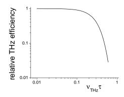
Fig. 2. Reduction factor  $g_1$  as a function of  $v_{THz}\tau$  for the case of femtosecond pump pulses ( $v_{THz}=\Omega/2\pi$ ).
