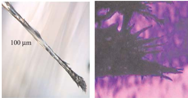
FIGURE 5 Evidence of self-focusing in lead silicate and chalcogenide glass
