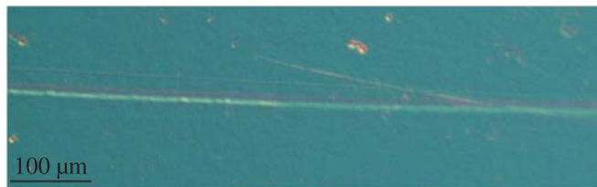
FIGURE 8 Waveguide fabricated with the unamplified Ti:Sapphire laser
