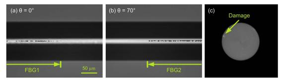
Fig. 7. Microscope images of UV-induced damages on the phosphate fiber cladding surface for (a) FBG1 with rotation angle  $\theta = 0^{\circ}$ ; (b) FBG2 with rotation angle  $\theta = 70^{\circ}$ ; (c) cross-section of a cleaved FBG.
