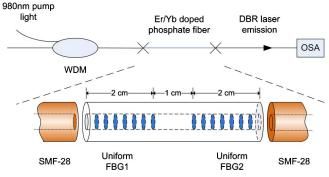
Fig. 1. Schematic of the short dual-wavelength singlelongitudinal mode DBR phosphate fiber laser.
