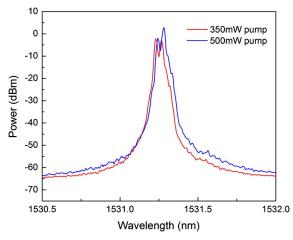
Fig. 3. Optical spectra of the dual-wavelength DBR phosphate fiber laser pumped at 350 and 500 mW.
