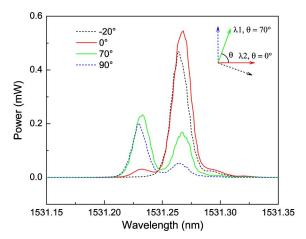
Fig. 6. Laser output spectra transmitted through a polarization analyzer at different angles. The inset shows the polarization states of two lasing lines ( $\lambda_1$  and  $\lambda_2$ : short- and long-lasing wavelengths).
