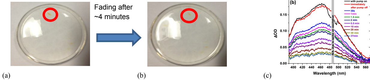
Figure 5: (a) Photo of the reversible color change of sol-gel disc samples due to excitation by a femtosecond pulsed laser at 620 nm resulting in photochromism induced by 2PA-FRET mechanism in the laser beam area (circled). (b) The color fades in ~4 minutes as a result of a thermally reversible process. (c) The obtained spectrum of the "open-ring" derivative peaking at 460 nm and its decay with time.
