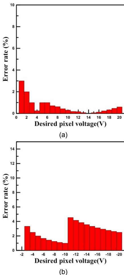
**Figure 4.** Simulated stored voltage error rates of proposed pixel circuit with different desired operation pixel voltages. (a) Positive polarity and (b) Negative polarity.
