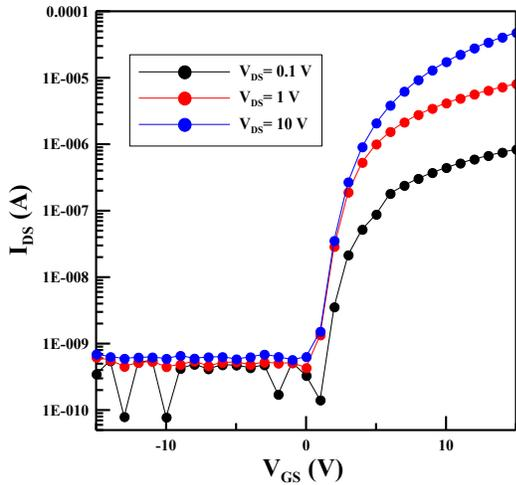
**Figure. 2.** Transfer characteristics of a-IGZO TFT with  $W/L=40 \mu\text{m}/ 10 \mu\text{m}$
